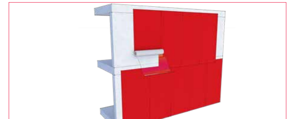
Fig.3 Staggered vertical installation of Wraptite membrane.
