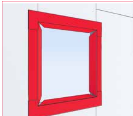
Fig.8c: Wraptite Tape cut at 45deg angles and folded inwards.
